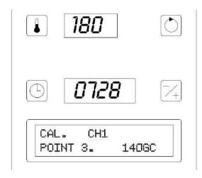
In the clear type display POINT 3. for the calibration is requested. Adjust the temperature of the third resistor in the temperature display using the encoder.
