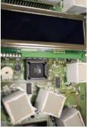
Put the new FLASH (that includes the software-update) into the socket.
