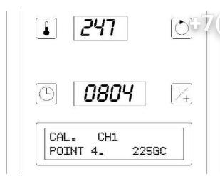
In the clear type display POINT 4. for the calibration is requested. Adjust the temperature of the fourth resistor in the temperature display using the encoder.
