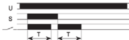
FZ11: Signal ON pulse + OFF pulse
