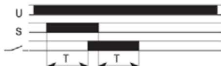
FZ12: Signal ON and OFF delay
