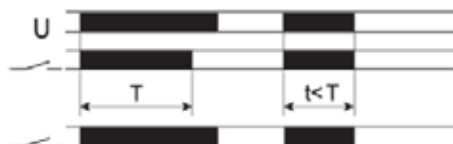
FZ19: ON pulse (1 timed contact + 1 instantaneous contact)
