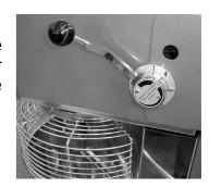
7. When the ingredients have been thouroughly mixed, press the stop button. Lower the bowl by pushing the bowl lift lever back and down to its resting position. Rotate the bowl guard so that it is in the open position. Rotate the tools anticlockwise for unhooking it and use levers to take the bowl with the tool out.
