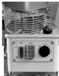
5. Press the main button (see pos.1 of the exploded view). Rotate the timer (pos.3) into ON position so to have a continuous
