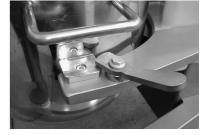
3. Rotate the bowl guard so that it rests in the open position and lower the bowl in its resting position. Select the appropriate tool and insert it onto the tool shaft. Move the agitator so that the notch on the agitator fits over the pin on the tool shaft as shown in the figure.
