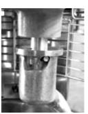
4. Lift completely up on the bowl lift lever until it locks into position. Insert the ingredients into the bowl and start the mixing process.
